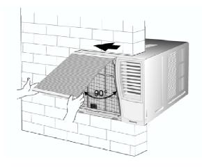
Caution: Do not raise the front intake grille any higher than  $90^{\circ}$  to the unit or damage to the tabs may occur.
